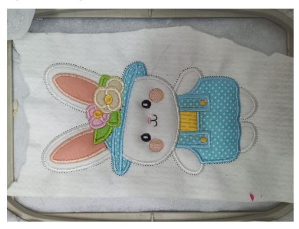
STEP 6: Remove the hoop from the machine and attach with tape a felt piece to the back
