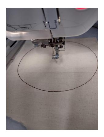
STEP7: Stitch the appliqué part and Stitch the placement line for the pocket
