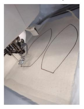
STEP 3: Stitch the appliqué step and place the fabric on the top of the hoop and Stitch it
