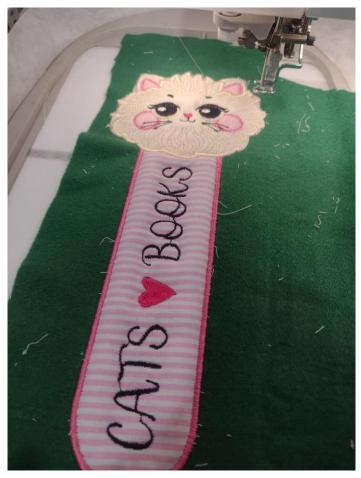
STEP 6: Before the last machine step, remove the hoop from the machine and attach with tape a felt piece to the back
