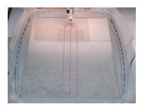
3-Place closed zipper (face up) over the placement lines, so that the coil lies on top of the center.
