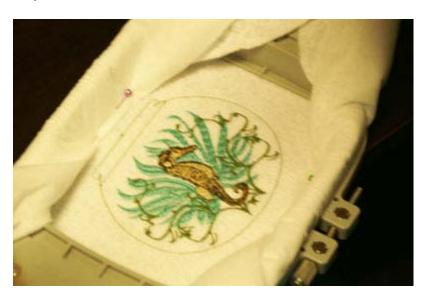
Take the <u>hoop</u> out of the <u>machine</u> and secure a 4×4 piece of clear vinyl on top of the design, making sure that the vinyl extends past the edges of the fishbowl.
