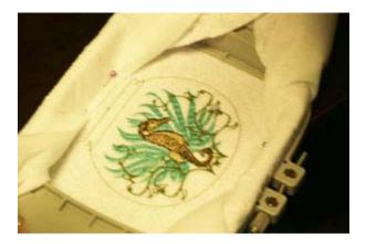
Place the <u>hoop</u> back into the <u>machine</u> and sew the next stitch, this will be the zigzag that will sew the vinyl securely in place.
