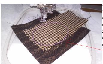
3-Lay center applique fabric over placement lines and stitch next color. I almost missed the bottom edge here. It really doesn't matter, another piece of applique is going over it. If not I would have ripped it out.
