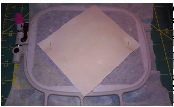
6-Remove hoop from machine and add the backing. I only used 2 pins, one at the top and one at the bottom, to hold the backing in place. Check as you put the hoop back on the machine to make sure nothing wrinkled up. Stitch the last color and button holes.
