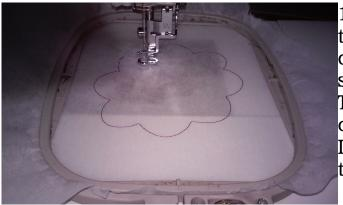
1-Hoope your stablizer and stitch the first color, lay the front fabric down over stitching lines, make sure the lines are complety covered. This picture looks like something is on the hoop, its not. It's the light from the camera and the machine
