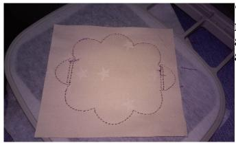
7-Remove hoop from machine and material from hoop and trim around the edges, again leave about 1/8".
